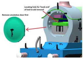
PCB), pull out the decoder PCB. When the PCB is fully removed from the smokebox the decoder blanking plate can be removed in the usual way.
